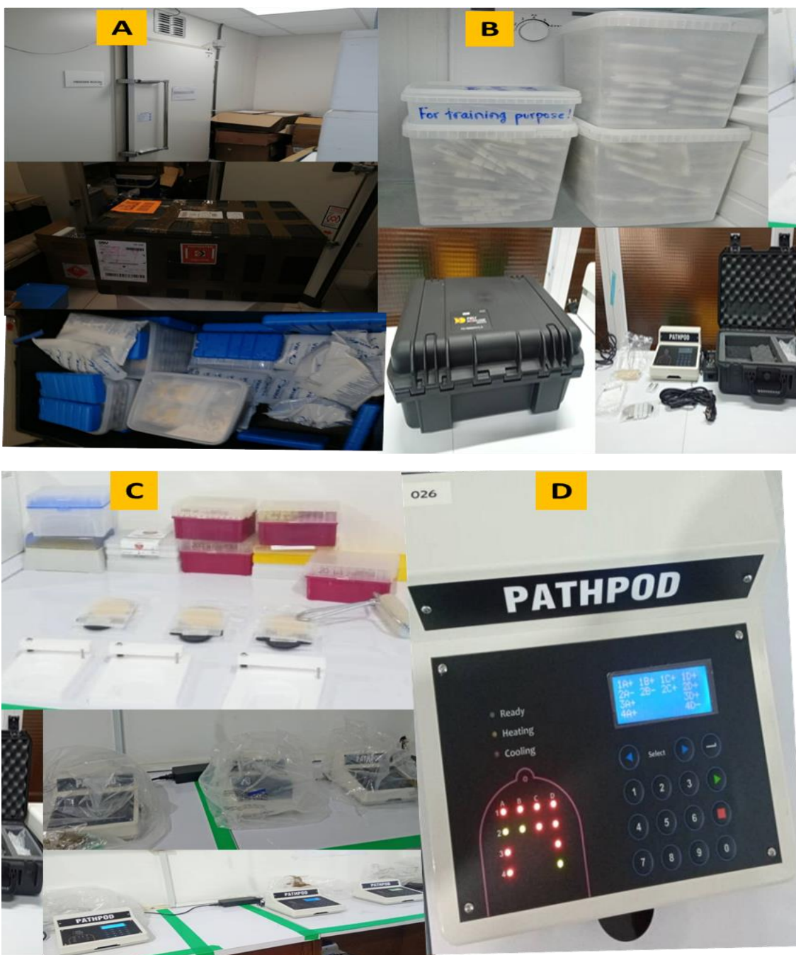
Figure 16: Nucleic Acid Testing system: a) Cold room storage of chips at NMIMR. b) Storage of chips at 4°C and storage of PATHPOD at KNUST. c) Chips and PATHPOD on the working bench. d) PATHPOD displaying
